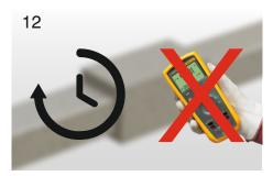
Megger test should not be conducted for a minimum of 24 hours after the casting process.
