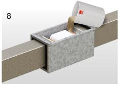
Alloy shall be casted uninterruptedly from the same Vibration is provided by means of plastic hammer.
