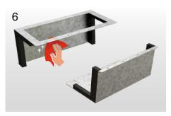
Inner surfaces of molds (surfaces subject to casting process) shall be cleaned with a clean and dry piece
