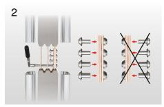
As shown on the figure, junction plates fixed as the bolts face the same direction at all times.
