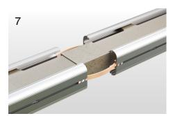
After the curing of the cast material is completed the sheet metal moulds can be removed. (Reaction is completed within 8 - 24 hours based on the air temperature.) The flexibles are fitted to the profiles grooves for earth continuity.
