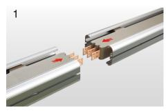
The ends of the conductors of the busbars are cleaned with a clean dry cloth. The busbars have to be fixed in the same axis, with a max. distance of 10 mm between the two conductors.
