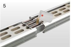
The mixture prepared for casting should be cast from the same spot at all times.
