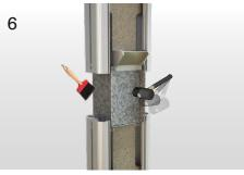
The material should be "vibrated" with the help of a plastic hammer to remove the air in the material. Then the air bubbles on the surface have to brushed.
