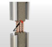
All bolts must be tightened to 72 Nm with torque wrench.
