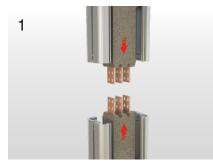
The ends of the conductors of the busbars are cleaned with a clean dry cloth. The busbars have to be fixed in the sameaxis, with a max. distance of 10 mm between the two conductors.
