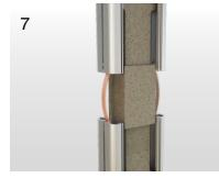
After the curing of the cast material is complete the sheet metal moulds can be removed. (Reaction is completed within 8 - 24 hours based on the air temperature.)The flexibles are fitted to the profiles grooves for earth continuity.
