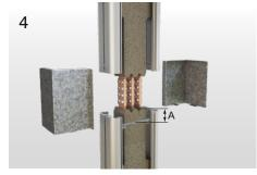
Support sheets are secured on the lower part of juncture area by stem bar. A min. 50-60 mm. The joint moulds are affixed on the support sheet by cleaning with a dry and clean piece of cloth.
