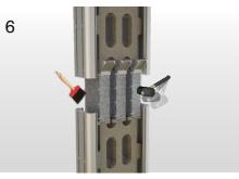
The material should be 'vibrated' with the help of a plastic hammer to remove the air in thematerial. Then the air bubbles on the surface have to brushed.
