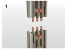
The ends of the conductors of the be busbars are cleaned witha clean dry cloth. The busbars have to fixed in the sameaxis, with a max. distance of 10 mm between the two conductors.
