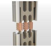
As shown on the figure, junction plates shall be fixed as the bolts face the same direction at all times.
