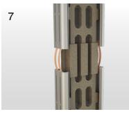
After the curing of the cast material is complete the sheet metal moulds can be removed. (Reaction is completed within 8 - 24 hours based on the air temperature. )The flexibles are fitted to the profiles grooves for earth continuity.
