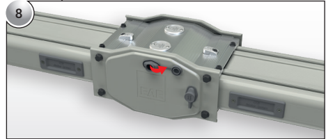
8 Plastic lid of the pouring area is removed. Attention! Pouring is done through the lid that is positioned on the upper side according to the busbar position direction.
