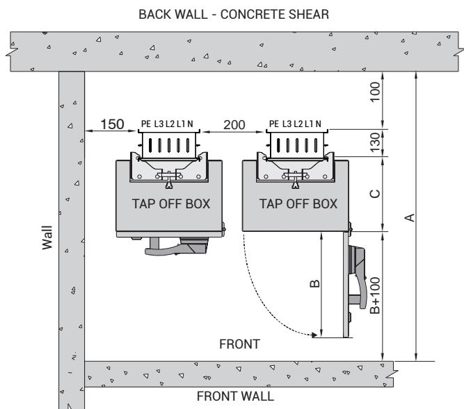
FIGURE-8 SHAFT LAYOUT DIMENSIONS (HORIZONTAL)
