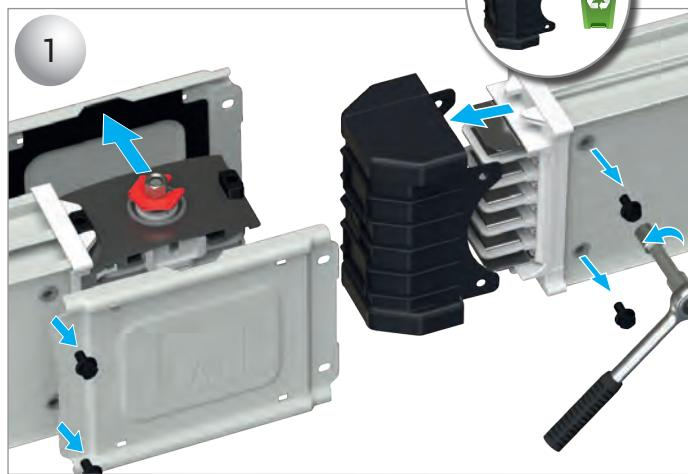
1- Align the body with and without block adjunct. Remove the adjunct cover and protection plastic.
