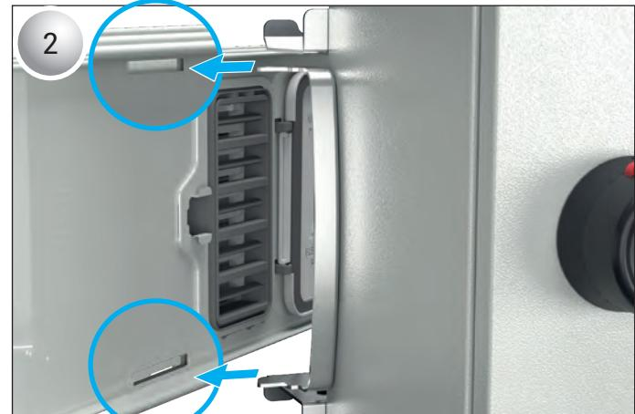
2- Insert the box lever plate to the handle hole on the body.
