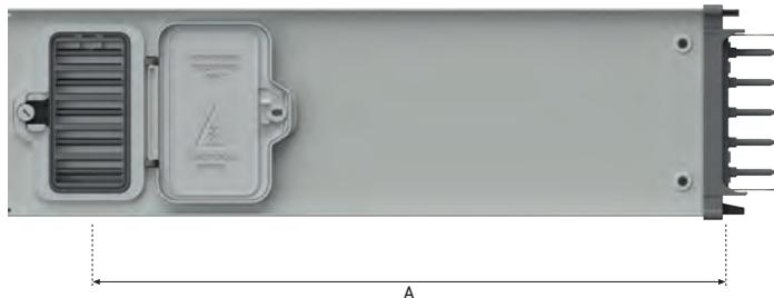
**NOTE:** A Min. in the Sheet Metal Boxes is the dimension of the position of Sheet Metal Boxes that is aligned with the groove on the full axis of Adjunct, as shown in Figure-2. If A Min. cannot be aligned with the groove on the Duct Adjunct, it should be 130 mm. less than (A Min) as shown in Figure-3.
