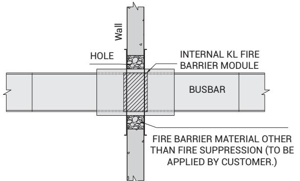
FIGURE-5 EXAMPLE WALL PASSAGE WITH FIRE BARRIER
