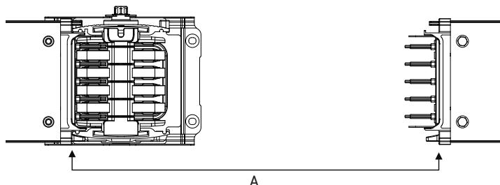
The dimension X is the measurement in cm from the corner of the body plate of a busbar to the other busbar's corner of body plate. Then, by subtracting 120mm from this dimension, midsize dimension is calculated.
